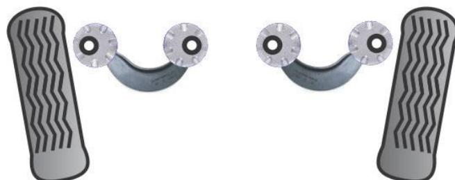
Sleeves adjusted to give maximum positive camber
