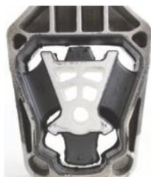
Figure 2 - The lower engine mount
