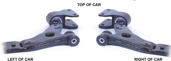
Figure 4 - Right-hand and left-hand bush and bracket assembly
